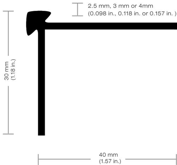
This aluminum nosing is a clean and simple design solution. It improves the overall quality of the installation by protecting the cement nosing, which is the weakest part of the stair construction and the area most affected by traffic.
