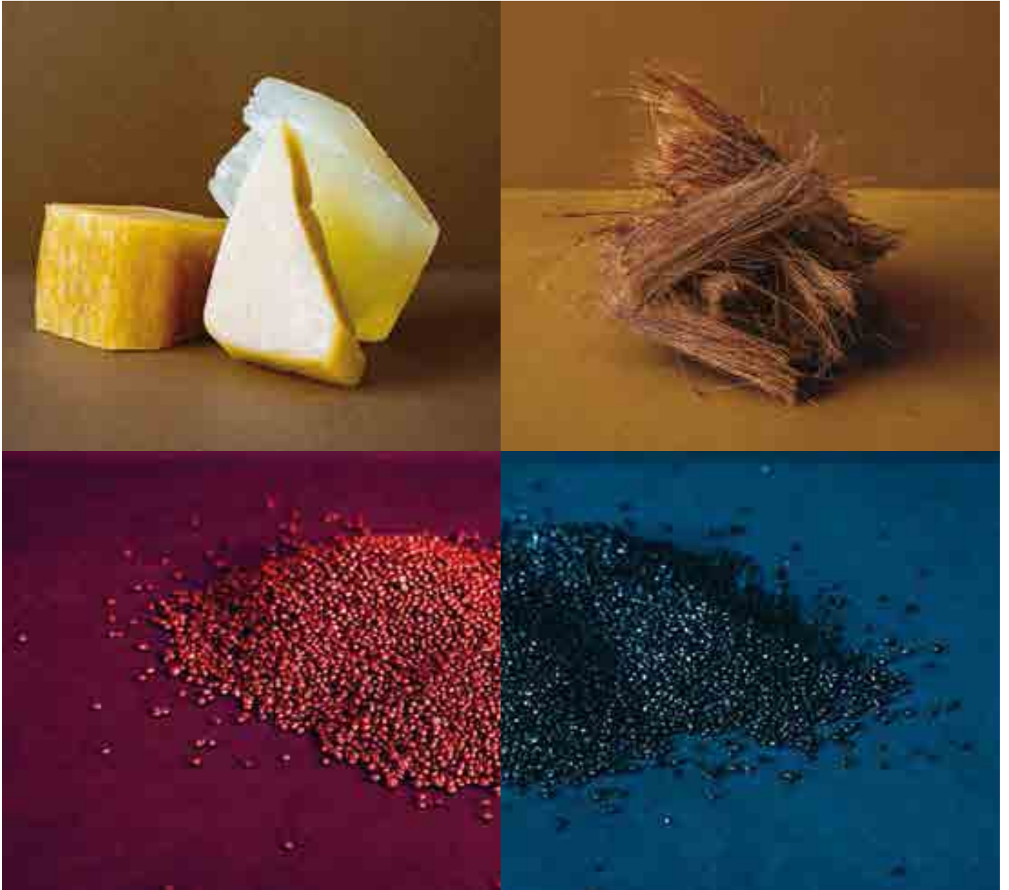
Raw and synthetic rubber, coconut fibers and color pigments used in the production of Mondo Rubber Flooring.
